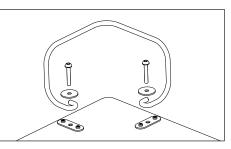
**NOTE:** Use only a manual screwdriver to install the retainer bolts. DO NOT use a power screwdriver to tighten the bolts.
