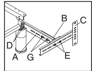
7. Measure the distance of the center to center mounting holes in the headboard.
