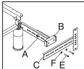
5. Ensure the headboard bracket is assembled a distance of 1.5 (38.1 mm) to 2 inches (50.8 mm) between the edge of the power base and the headboard bracket assemblies.
