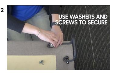
Secure the retainer bar using the allen wrench provided.
