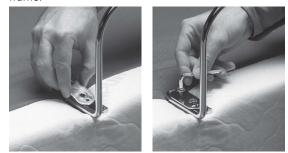
NOTE: Use ONLY a manual Allen Wrench to install the Retainer Bar Bolts. DO NOT use a power tool to tighten the bolts. DO NOT over tighten the mattress retainer hardware!
