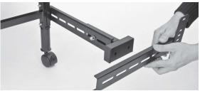
Place Bracket Bolts (D) with a 5/16 inch washer (F) through the Outer Headboard Bracket (C) and into the Inner Headboard Bracket (B). Use 5/16 inch washers (F) and 5/16 inch nuts (G) and hand tighten to allow for adjustment.
