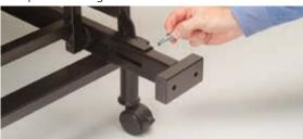
Adding the 5/16 inch washer (I) and 5/16 inch nut (J), hand tighten the bolt in place using the supplied wrenches (K and L).
