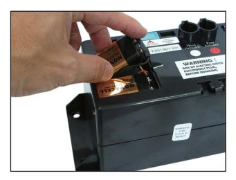
Figure 2: Install 9 volt batteries.
