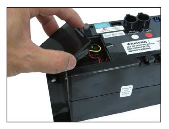
Figure 1: 9 volt batteries cover.
