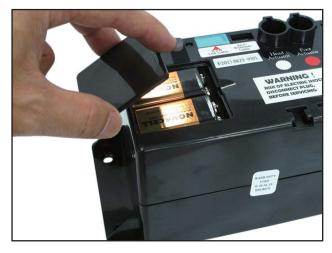
Figure 3: Replace battery cover.
